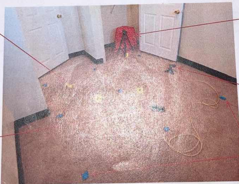
Photo #5 (THB 2/14/20). Floor grid illuminance test setup.
