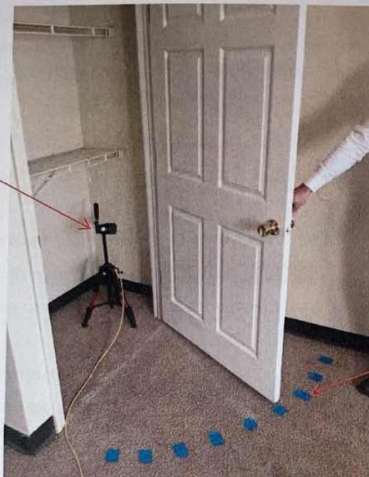
Photo #8 (THB 2/14/20). Door closure angle illuminance test setup.
